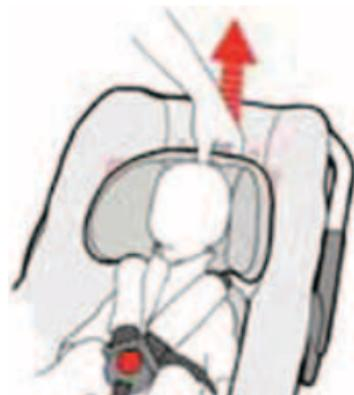
Release the switch and move the headrest until it reaches the nearest locking position, when you should hear a click. Check that it is locked by pulling the headrest.
