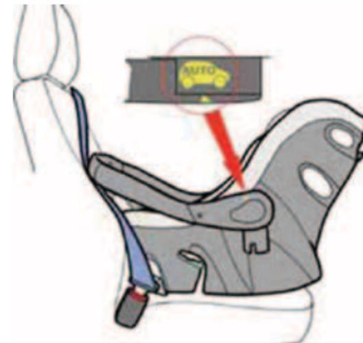
Pass the abdominal part of the car seat belt through the front slots (01) on the side of the casing.
