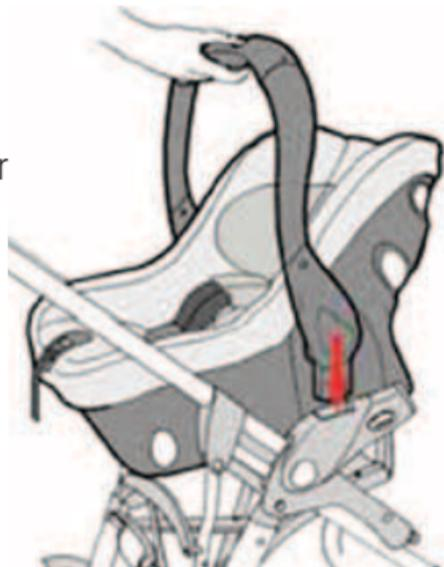
To release your CONCORD INTENSE from the chassis, press the switch (11) on the handle and pull the seat upwards.
