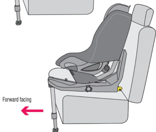
Extract the ISOfix anchors (6) by turning the handle (9) on the side of the base. The anti-rotation leg (12) will unfold due to IKONIC R. ①.a
